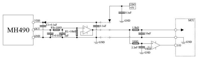
For proper operation a 100nF or bigger bypass capacitor C1 should be placed as close as possible to the VDD and GND pins, and a bypass capacitor C2 of 1nF to 10nF can be placed on the output of MH490.
