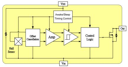
*Note:* Static sensitive device; please observe ESD precautions. Reverse  $V_{DD}$  protection is not included. For reverse voltage protection, a 100 $\Omega$  resistor in series with  $V_{DD}$  is recommended.
