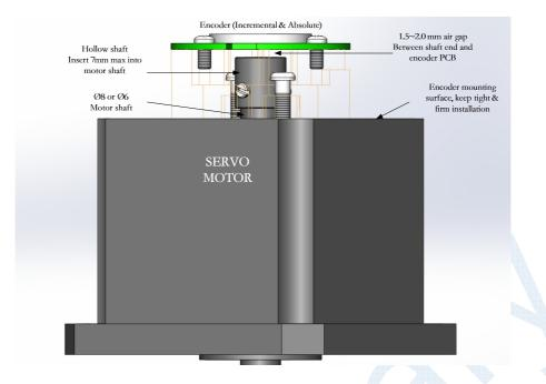
After coupling the encoder hollow shaft with the rigid motor shaft, always fasten attached screws securely. Be sure to firmly tighten two hex-screws that located at encoder's hollow shaft, apply threads-lock glue and tightly screwed in for long-term use. Also follow above procedures for the encoder M3 screws when mounting the encoder onto servo motor.
