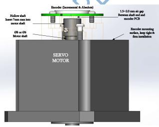
After coupling the encoder hollow shaft with the rigid motor shaft, always fasten attached screws securely. Be sure to firmly tighten two hex-screws that located at encoder's hollow shaft, apply threadslock glue and tightly screwed in for long-term use. Also follow above procedures for the encoder M3 screws when mounting the encoder onto servo motor.
