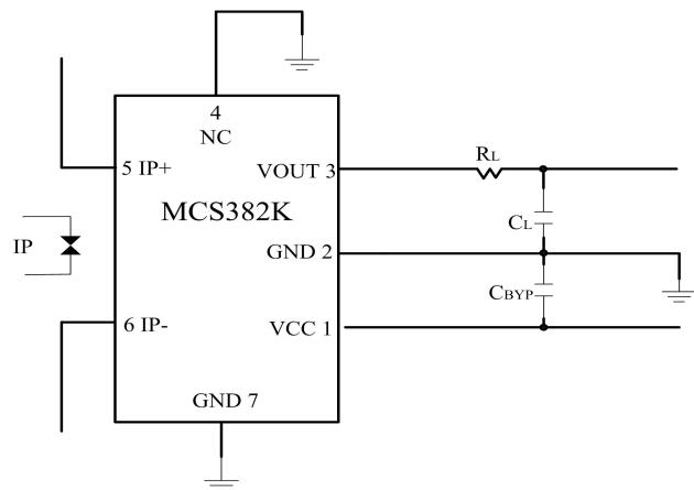
\*If the application circuit power supply (Vcc) may have a transient pulse spike greater than 6.5V, it is recommended to add TVS tube between Vcc and GND to absorb the spike energy.
